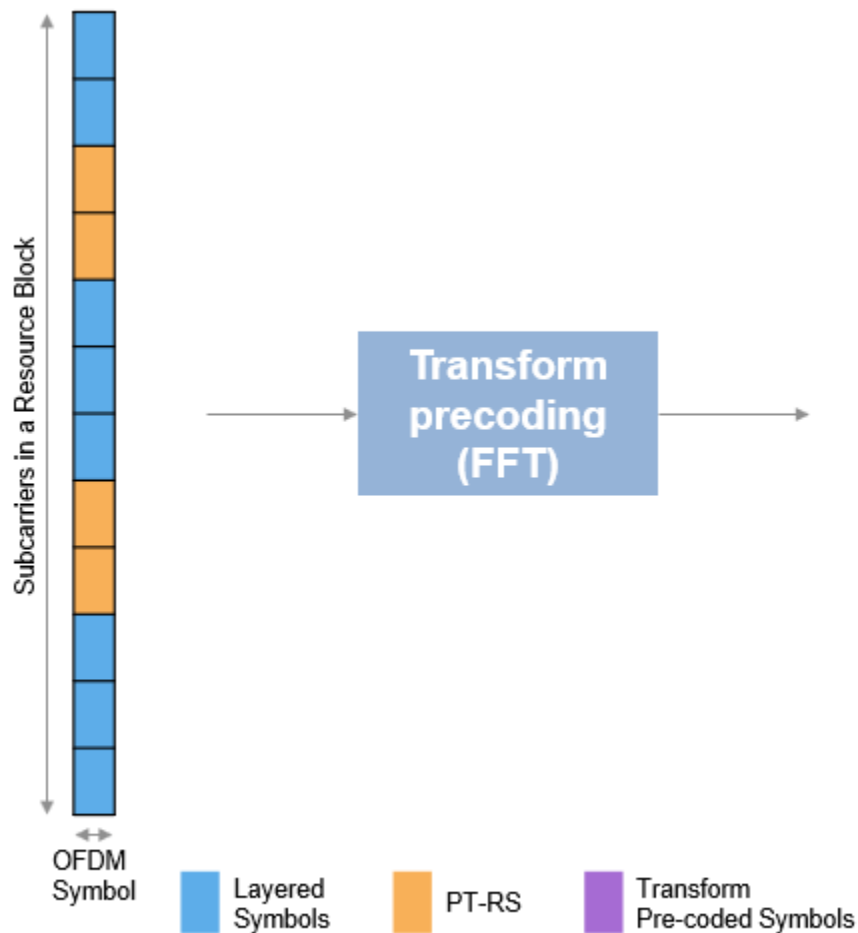
Figure 3: PT-RS Insertion in DFT-s-OFDM
